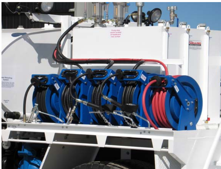
Multi-compartment tank with sight tubes, lockable fill caps. Oil tanks have filtered vents.
