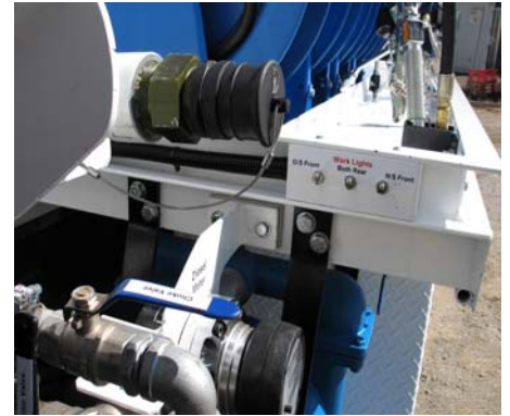
Diesel is dispensed by 38mm air-operated diaphragm pump and measured through 38mm Macnaught flow-
