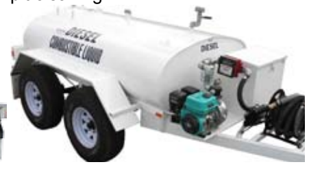
Conventional diesel trailers in 1k, 2k and 3500L versions. Reg'ble & unreg'ble with range of pumpsets
