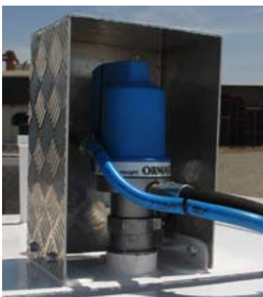
Macnaugh T512 5:1 ratio oil pump with protective guard.
