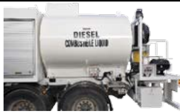
Diesel tanks for service trucks
