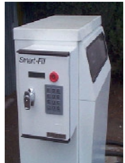
This image shows a Smart-Fill system installed to a mechanical fuel bowser (Fleet-line T334 hi-flow diesel). The system may be installed to almost any mechanical fuel bowser.
